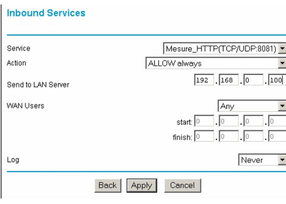
The screenshot shows the 'Inbound Services' configuration page. The 'Service' dropdown is 'Mesure\_HTTP(TCP/UDP:8081)', 'Action' is 'ALLOW always', 'Send to LAN Server' is '192.168.0.100', 'WAN Users' is 'Any', and 'Log' is 'Never'. There are 'Back', 'Apply', and 'Cancel' buttons at the bottom.
