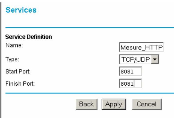
The screenshot shows the 'Services' configuration page. Under 'Service Definition', the 'Name' field is 'Mesure\_HTTP', 'Type' is 'TCP/UDP', 'Start Port' is '8081', and 'Finish Port' is '8081'. There are 'Back', 'Apply', and 'Cancel' buttons at the bottom.
